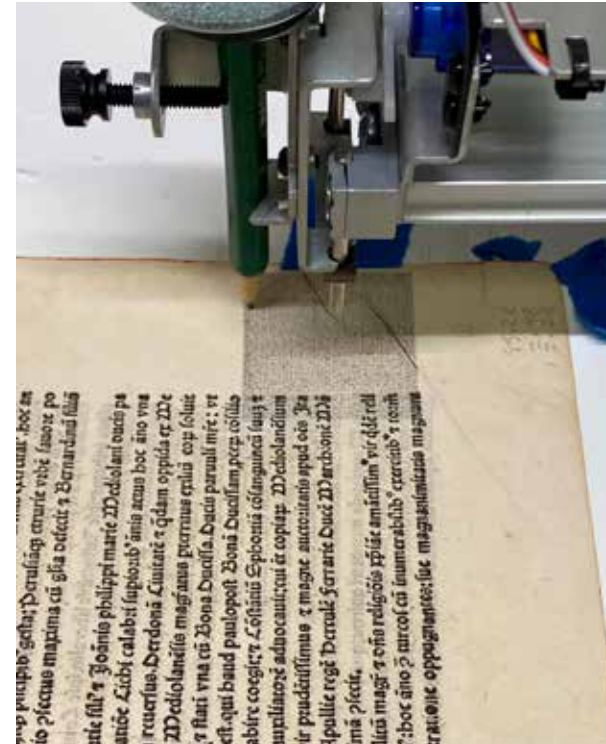
Magnolia Editions pencil drawing plotter 2B lead, .07mm, 41g pressure, 3.5 x 3.5 mm graphite
