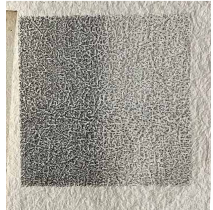
Magnolia Editions 2021 paper with felt hair marks 2B lead, .07mm, 41g pressure, 3.5 x 3.5 mm graphite
