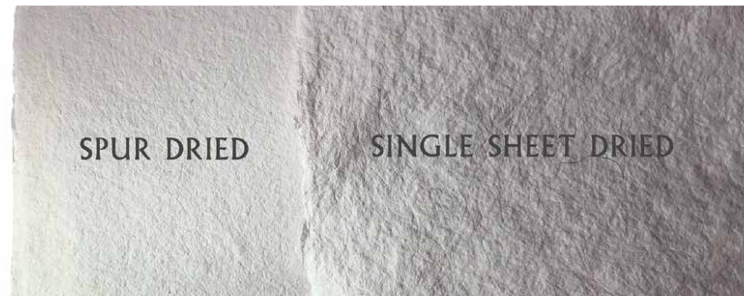
These two sheets were made with the same furnish—the texture difference is a result of constrained and unconstrained drying.
