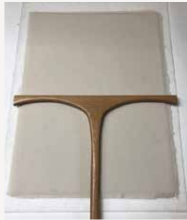
Step 1: place T off-center of pack. Note: wire side of paper (right side) is face up.
