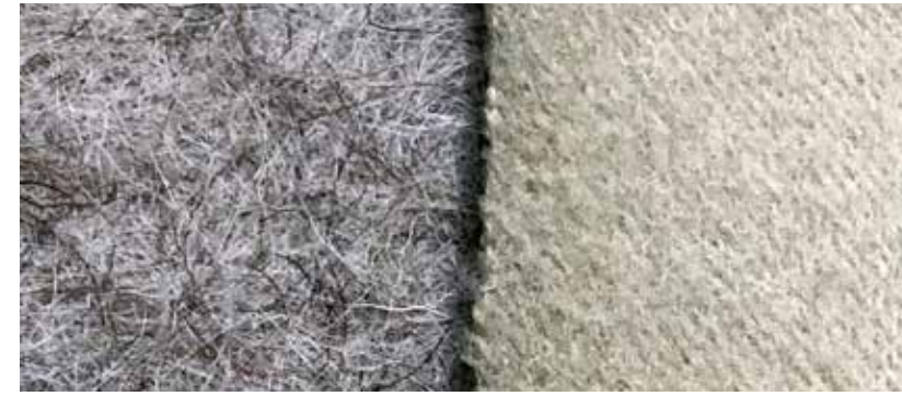
Churro handmade felt at left; an industrial woven and “needled” wool felt at right
