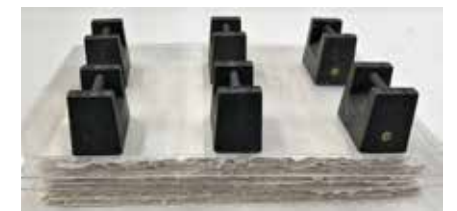
Curing under the pressure of 5kg weights
