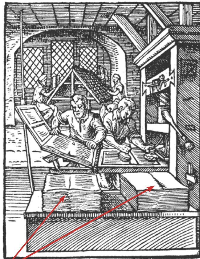
Figure 3. Jost Amman's 1568 woodcut depicting book printers (Book of Trades) clearly shows us the back mark in the unprinted and printed leaves in the foreground. The printers carefully place it in the gutter of the leaf.
