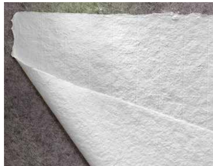
This air-dried, folded sheet shows the wire side (top) and the felt side (bottom) on a Navajo-Churro felt.
