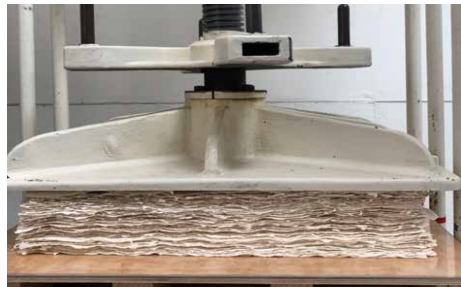
Finish pressing coaxes the cockled sheets flat over time
