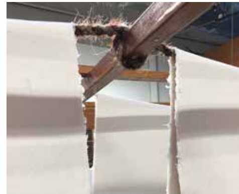
Spurs hanging/drying on treble lines—stretched horse-hair rope
