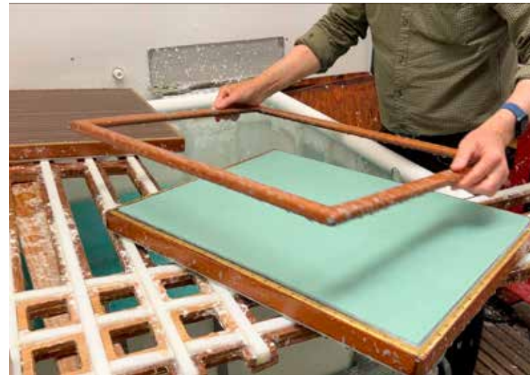
Lifting the deckle – transferring to empty mould
