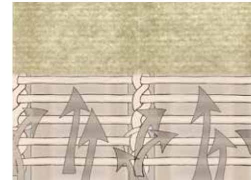
Figure 8: Furnish flow on the laid mould covering causes a heavier build-up of fibers washed to the drainage spaces (between the laid lines and on either side of the ribs). Those varied fiber densities generate the visible shadow of the laid lines and the thick/thin profile of “antique” laid paper.
