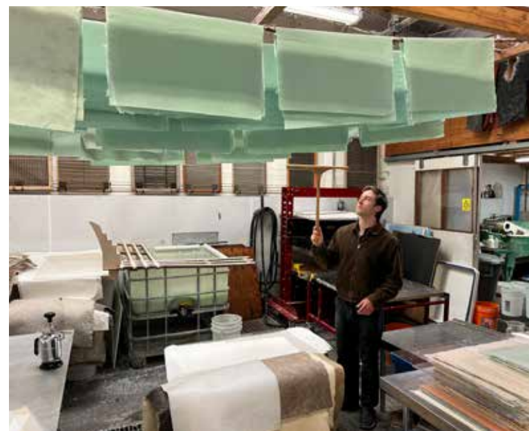
Hanging a spur on horsehair rope to dry using a "T"
