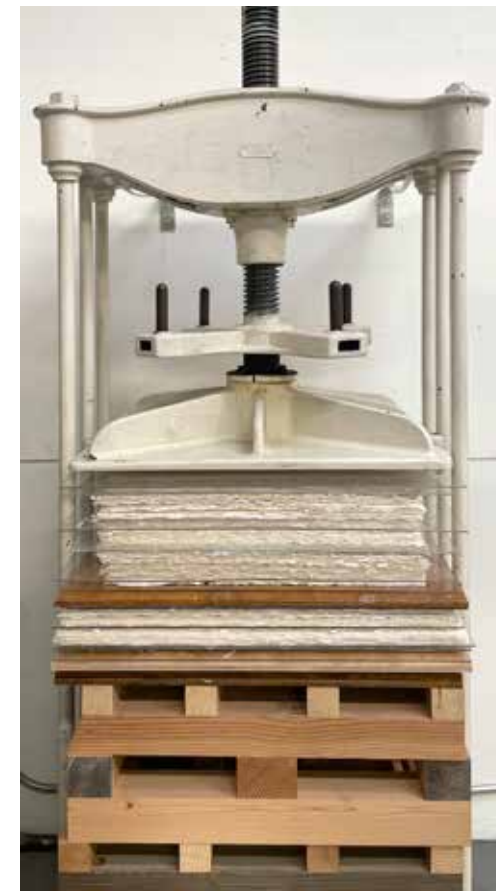
Greater pressure of a standing press used in the final stages of flattening
