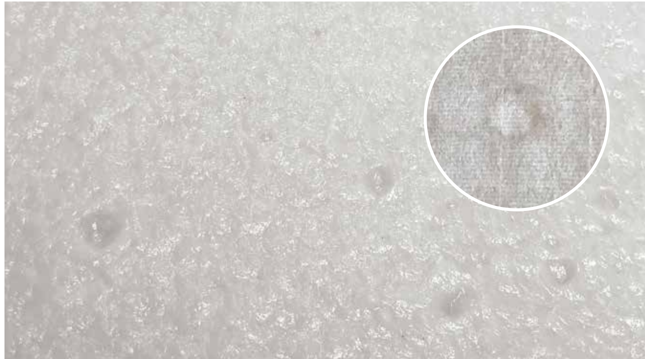
Vatman's drip marks made on the felt side while sheet is draining; inset, the same sheet after drying.
