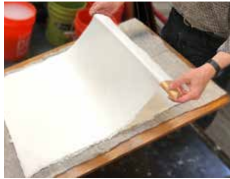
Placing a pressed sheet onto a pack
