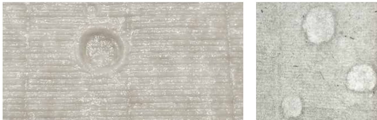
Coucher's drip mark on the wire side of a couched sheet; at right, a similar sheet after drying.
