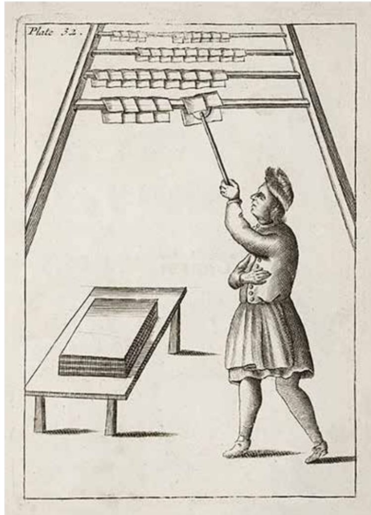
17th-century cartoon of a papermaker hanging sheets to dry, thereby leaving a back mark on each sheet
