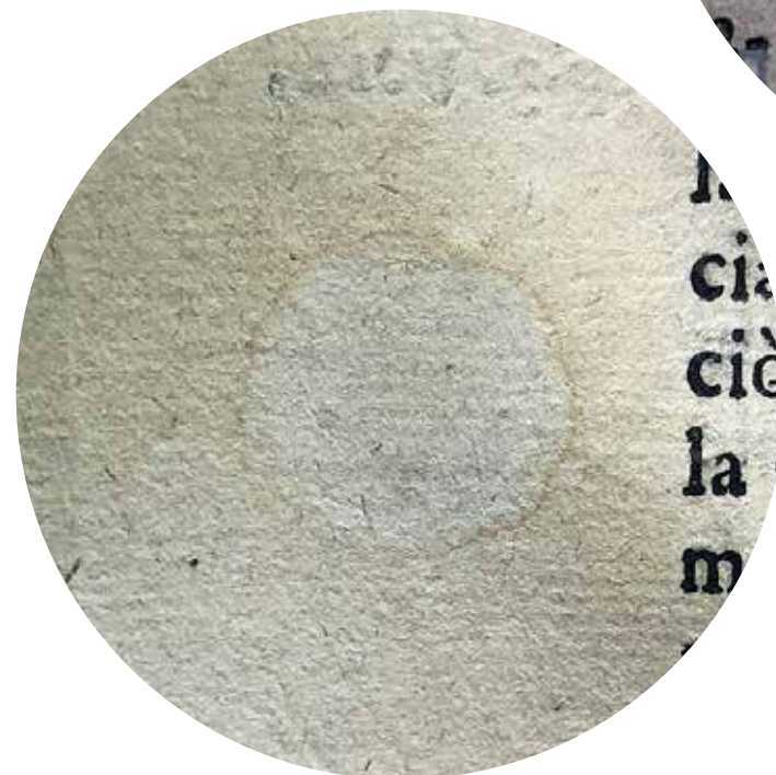
3. Verso, showing no fiber disruption nor crater dimensionality, is therefore the wire side, where the laid lines are still intact, the opposite side of the water's hit.
