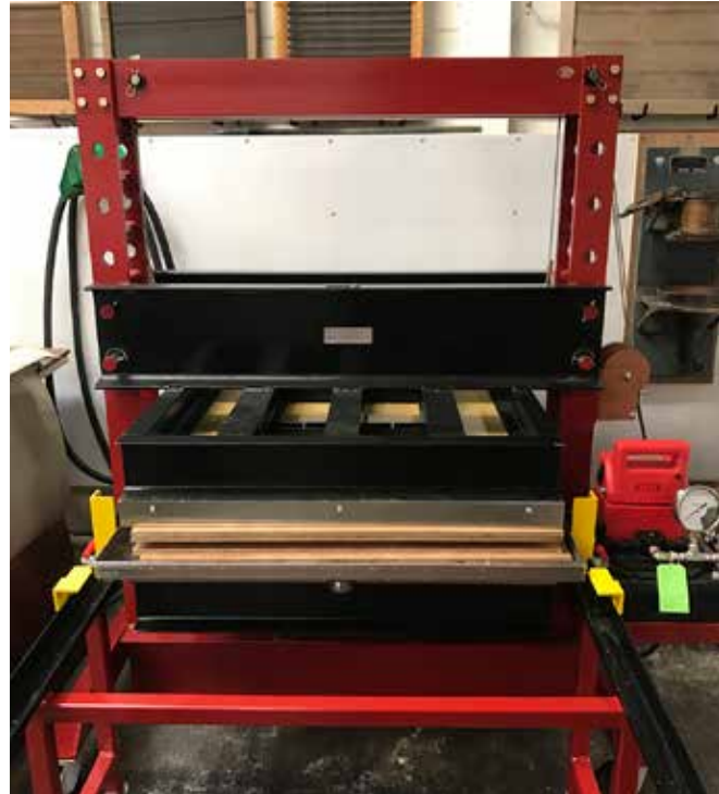
44 x 36 in. 50-ton hydraulic press
