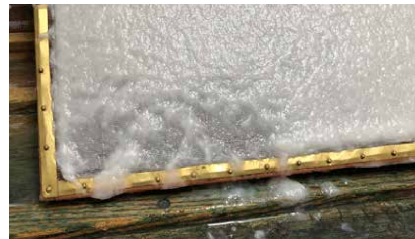
Slow (not free) furnish: needed more drainage time. This sheet was tilted on horn too early.
