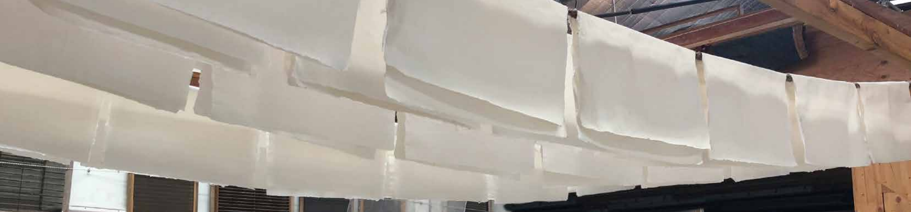
Paper hung to dry on horsehair rope suspended on a framework (“treble lines”)
