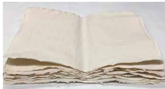
Spurs pulled down from drying ropes, separated, broken and stacked already demonstrate a good drape and conformity to the codex format
