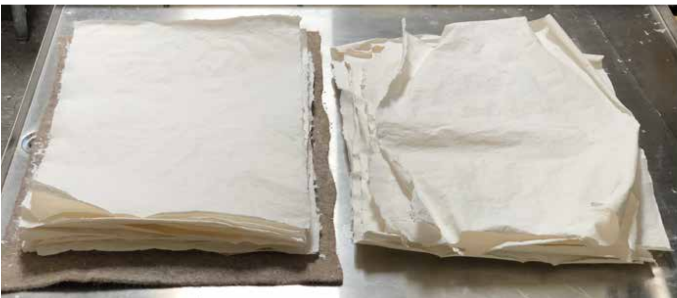
Papers dried individually, unconstrained. Sheets in the left-hand stack were dried on a moist felt; sheets at right were dried on treble lines and flat on taut screen drying rack.
