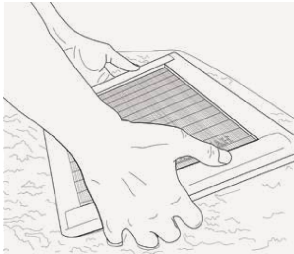
At the vat with mould and deckle, about to form a sheet
