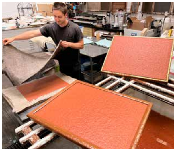
Laying aka pitching a felt
