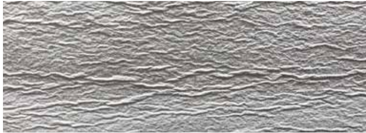
The convex topography of this back mark indicates it is the felt side.
